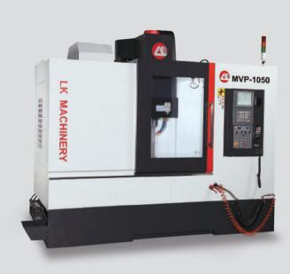
Direct Drive Spindle with 10,000rpm is the standard for MVP Series. Motor and spindle are connected by high precise coupling, and perform excellent transmission, display outstanding cutting.
